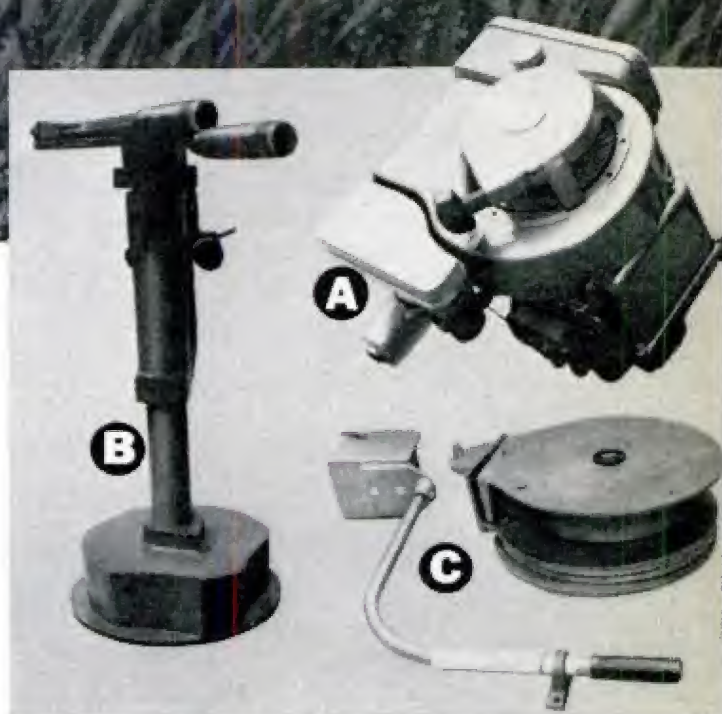
OUTBOARD (B) AND INBOARD (C) MODELS of Otterbine jet adapt to two or four-cycle engines. Author finds four-cycle system cleaner and prefers units such as the 8-hp Briggs & Stratton (A)
